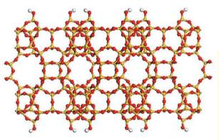
**Assembly required.** Porous zeolite crystals are widely used as filters and catalysts. This year, researchers found new ways to tailor the size of their pores and create thinner, cheaper membranes.
